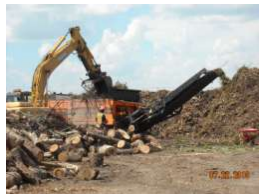
Shredding leaf and yard waste at the Saskatoon compost depot. Photo courtesy of the City of Saskatoon.
